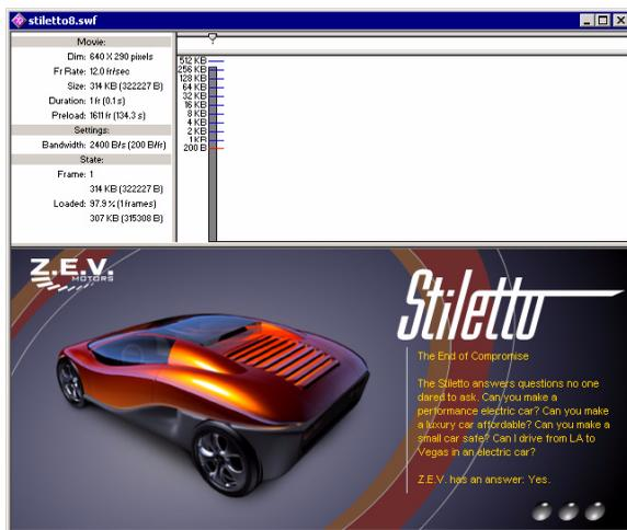
The shaded bar represents the first and only frame in your main movie. Movies with multiple frames will have multiple shaded bars. The height of the bar represents the frame's size in bytes and kilobytes. Bars that extend above the red line, especially if the bar represents a frame other than the first frame, indicate there could be delays in movie playback. You can optimize your movie for faster downloads. For details, see “Optimizing movies” under Help > Using Flash.
